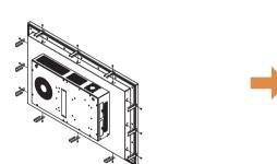
Step 2. Mount SP-S214 Panel PC equipped with 12 brackets onto the wall firmly.
