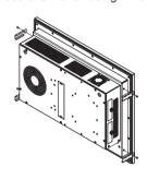
Step 2. Mount SP-S154 Panel PC equipped with 4 brackets onto the wall firmly.
