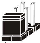
Jumper Block 1-2 pin close(enabled) Looks like this
