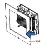
Step 2. Mount SP-6550 Panel PC equipped with 9 brackets onto
