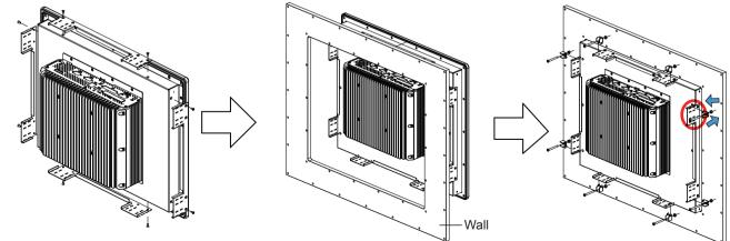
SP-6267 & SP-6269 Step 2. Mount SP-6267 & SP-6269 Panel PC equipped with 8 hooks onto the wall firmly.
