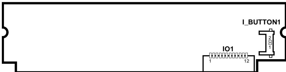
Figure 2-6. MB-3012 MSR Board Component Locations
