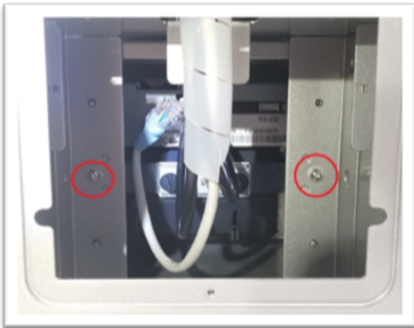
Step 19. Follow the cable labels and connect the cables with a head unit (Panel PC).
