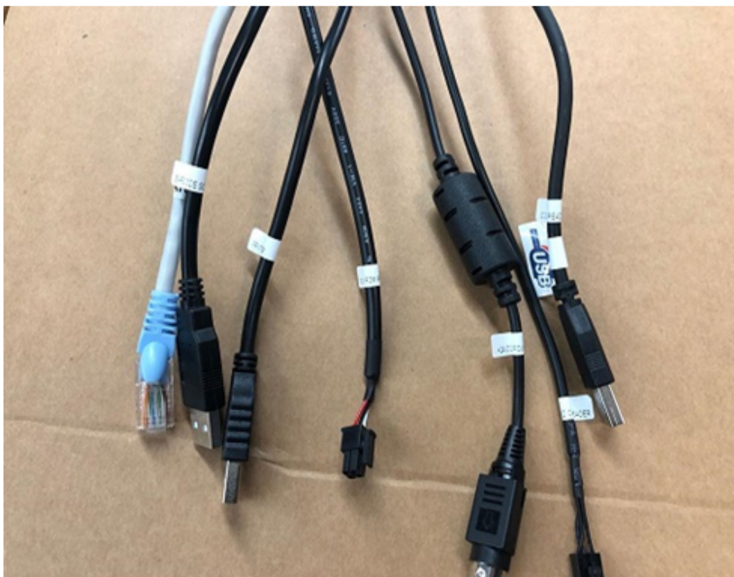
Step 19. Follow the cable labels and connect the cables with a head unit (Panel PC).
