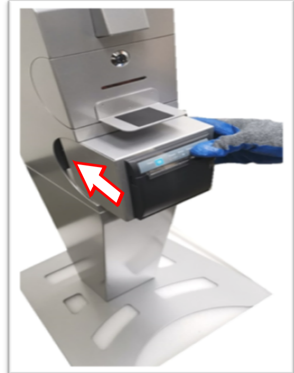
Step 18. Connect power cord to complete KIOSK stand installation.
