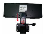
**Step 6.** Stretch out the VFD cable and then connect with the VFD Module cable.
