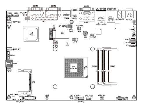
POS-6511 Mainboard Front Connector, Jumper and Component locations
