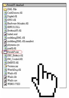
**Note:** (1) .Net Framework 2.0 or above must be installed on the operating system before running the API program, and (2) do not remove any file under the "ProxAPI standard" folder.
