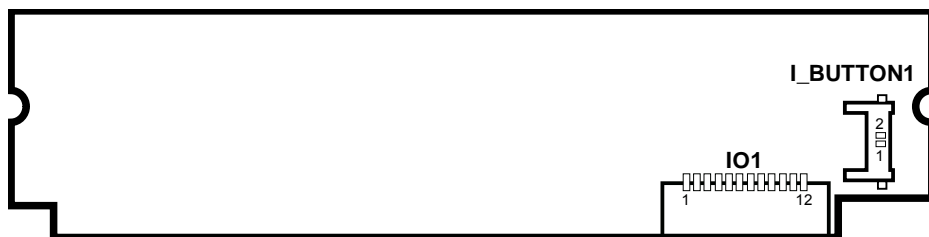
Figure 3-6. MB-3012 MSR Board Component Locations
