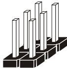
Jumper Block looks like this
