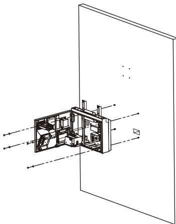
**Step 6.** Install the back cover of KDS onto the rear of KDS.
