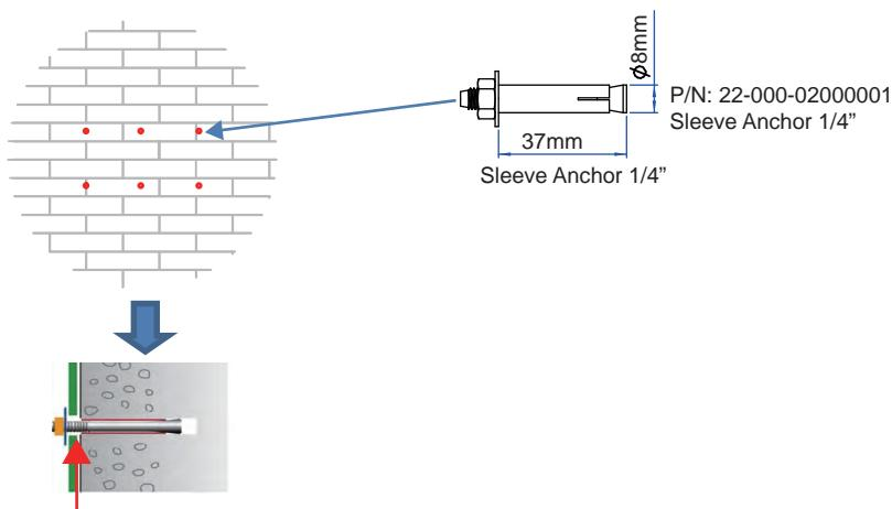
The sleeve part should be hidden into the wall.
