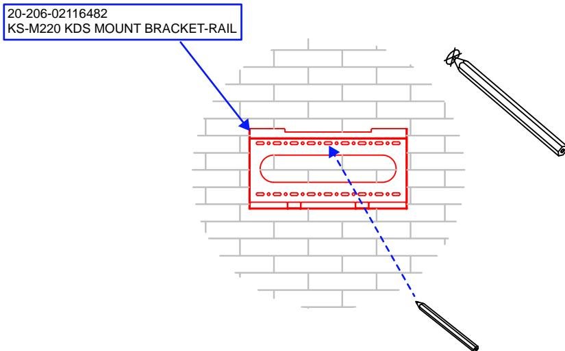
**Step 2.** Install the sleeve anchors into the intended locations. Note that the sleeve should be installed inside the wall.
