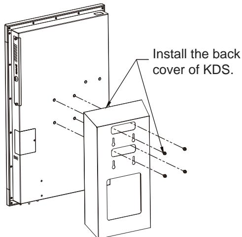
**Step 7.** Attach KDS onto the body.
