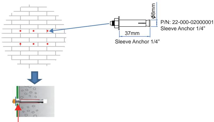
**Step 3.** Fix the KDS mount bracket-rail onto the wall:
