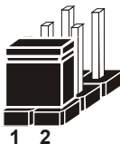
Jumper Block 1-2 pin close(enabled) Looks like this
